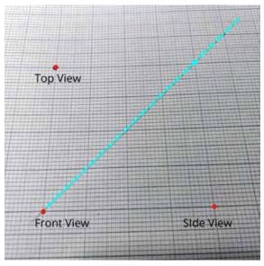
larger squares and mark another point - this will be the centre of your right side view. Go back to the front view and go up by 4 of the larger squares and mark a point for the centre of your top view. If needed, use a dash / dot line to connect these, for clarity.
